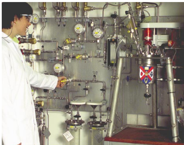
Dr. Sarah Thompson (née Boyle; EPSRC Clean Synthesis Fellow) with an autoclave for preparing ionic liquids
